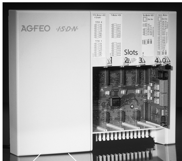
Figure 1: telephone system with detached cover
